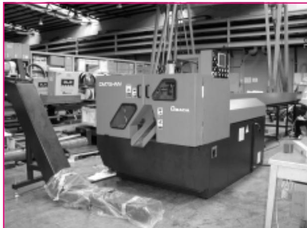
**A**mada’s new CM75AN-CNC uses a disposal circular carbide blade instead of a conventional bandsaw blade. It cuts all kinds of materials five to ten times faster than a conventional bandsaw and leaves a clean surface finish that seldom requires a secondary operation. ☎
