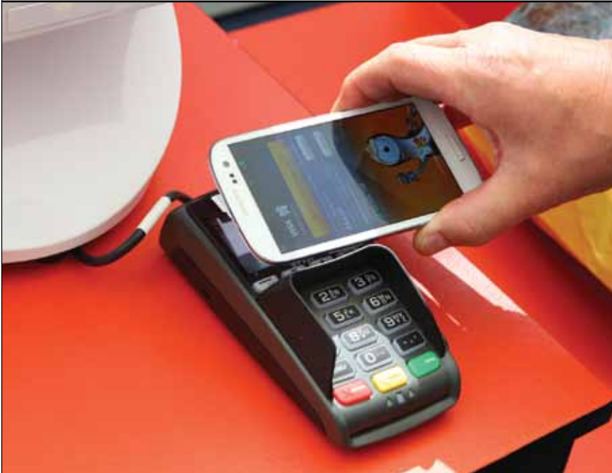
Figure 1. A Samsung smartphone makes a purchase via near-field communication, in which a user transmits payment information by placing the device close to a merchant's NFC reader.
